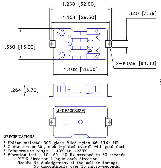
AUTH DR. CK. SYM REVISION RECORD Date ADDED "ROHS COMPLIANT" T.B. 11/05/05 ADDED PATENT NUMBER B.S. 2/11/06 DIMENSION .140 WAS .138 T.B. B.S. 2/17/07 ADDED SOLDERING SPEC. B.S. 4/26/08 6/27/08 MATERIAL WAS UL94V-0 T.B. B.S.
